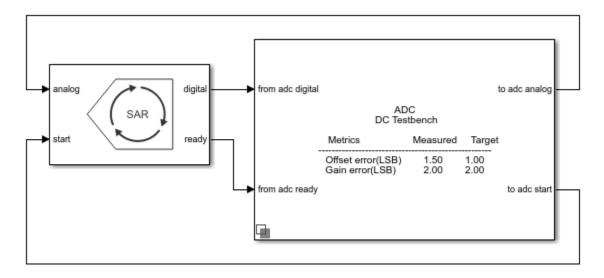
Double click the ADC Testbench block to open the Block Parameters dialog box. Click the **Plot DC analysis results** button to view the ADC transfer curve, endpoint nonlinearity and best fit nonlinearity.
