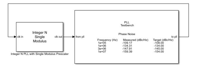
Double-click the PLL Testbench block to open the Block Parameters dialog box. Click the **Plot phase noise profile** button. The PLL operating frequency is 2.8 GHz, and the measured phase noise profile matches the target profile.
